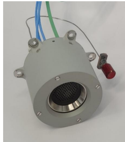
Figure 4. MSL's RIT3.5 Engineering Model.
