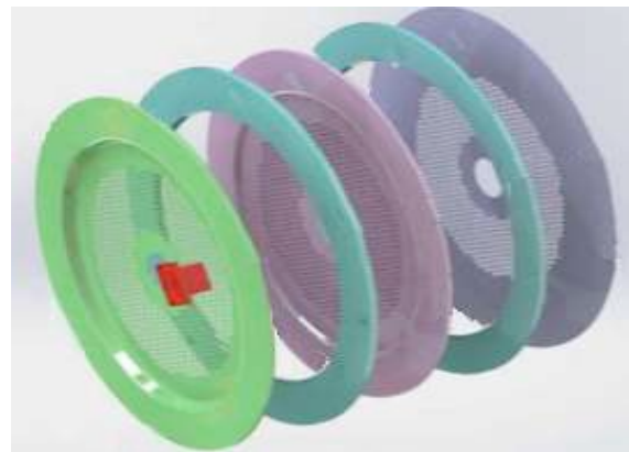
Figure 3: Ion Optic System sub-assembly of ITT: screen, accel and decal grids and spacers
