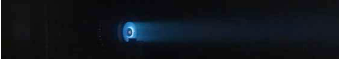
Figure 6: Impulse Transfer Thruster designed and manufactured by TransMIT GmbH running in DLR STG facility. Thrust \approx 28 mN; RF Power: 275 W; Mass Flow: 0.57 mg/s; Beam current: 290 mA; Drain current: < 2 %; Divergence: < 4^\circ ; Total power is under 1300 W.
