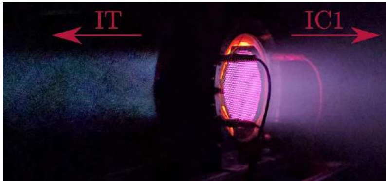
Figure 11. Extracted ion beams from the IT and IC1 ion optics systems in Configuration ADST.
