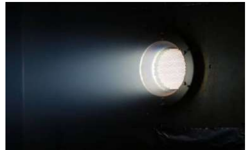
Figure 16. RIT-10 thruster running with O 2
