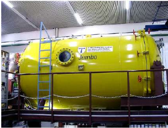
Figure 11. Vacuum test facility Jumbo
