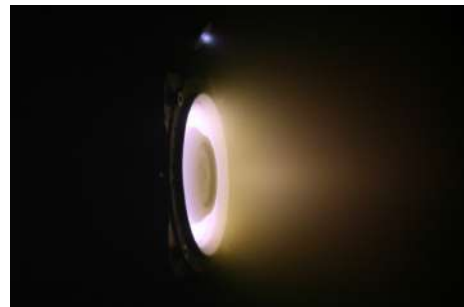
Figure 7. Thruster operating with N 2 /O 2 mixture (305 V, 2.75 mg/s)
